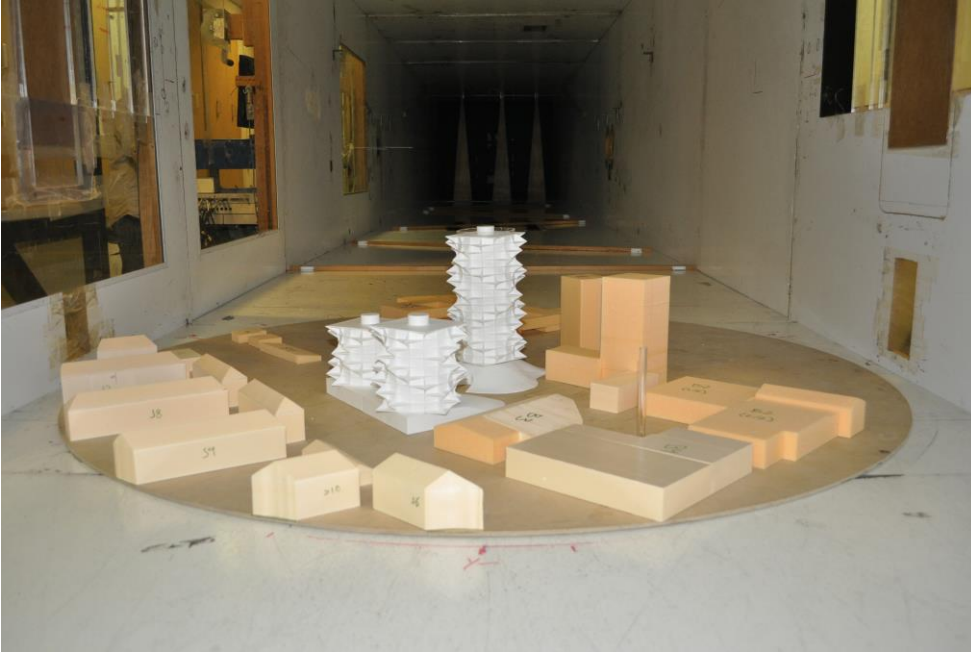
Figure 16. A Place To – Wind tunnel testing © Svend Ole Hansen ApS
