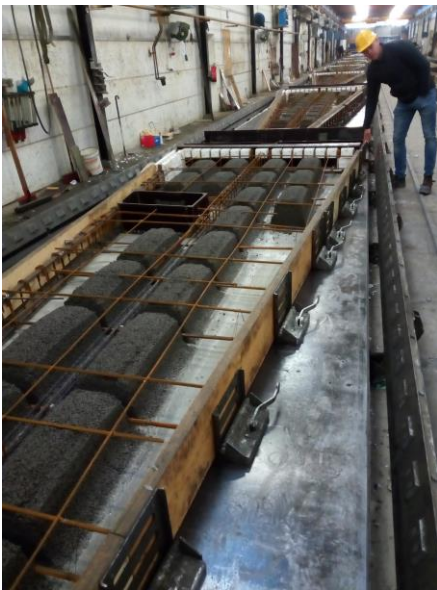
Figure 6. A Place To – SL-slabs during fabrication and installation © Abeo / A Place To
